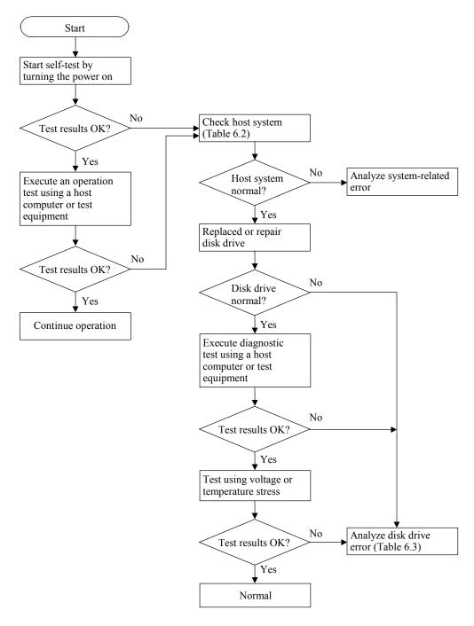
Figure 6.3 Test flowchart
